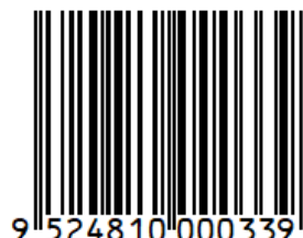
Figure 4-12 Example of EAN-13 with EAN/UPC HRI format
