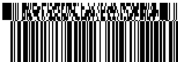
Figure 5-54 GS1-128 Composite symbol with CC-C
