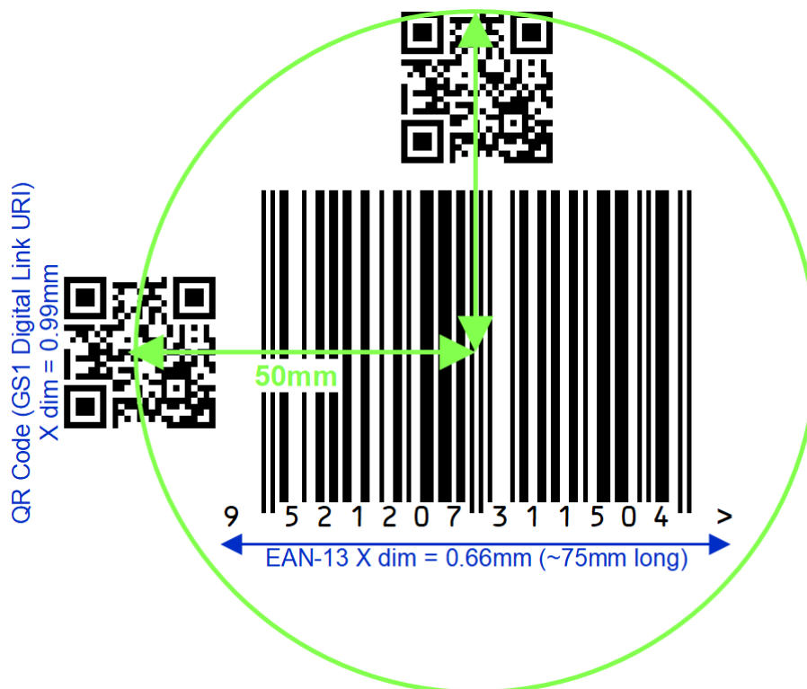
Figure 6-7 Maximum POS X-dimension 2D barcode placement in relation to the linear barcode example
