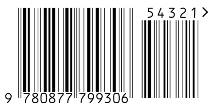
Figure 5-20 EAN-13 barcode with five-digit add-on symbol
