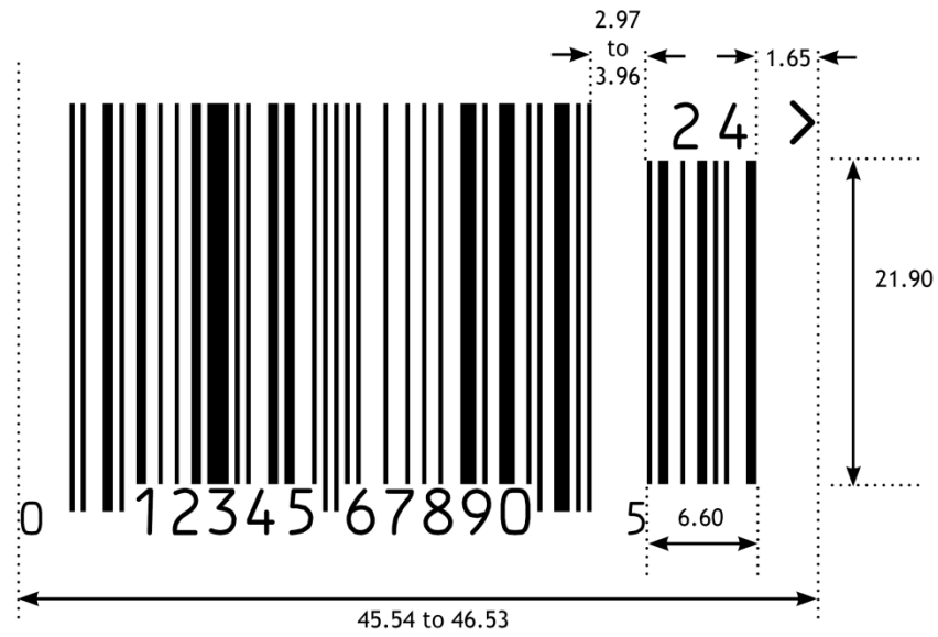
Figure 5-27 UPC-A barcode with two-digit add-on symbol
