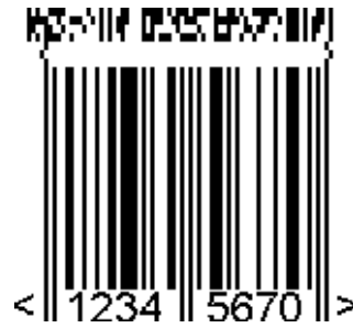
Figure 5-60 EAN-8 symbol with a three-column CC-A
