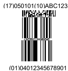
Figure 5-5 GS1 DataBar Stacked Omnidirectional barcode with a Composite Component
