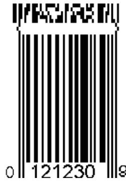
Figure 5-61 UPC-E symbol with a two-column CC-A
