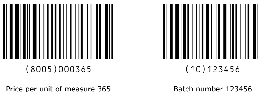
Figure 7-11 Data encoded in two GS1-128 symbols
