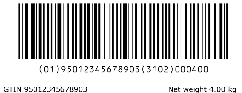
Figure 7-10 Data encoded in one concatenated GS1-128 symbol
