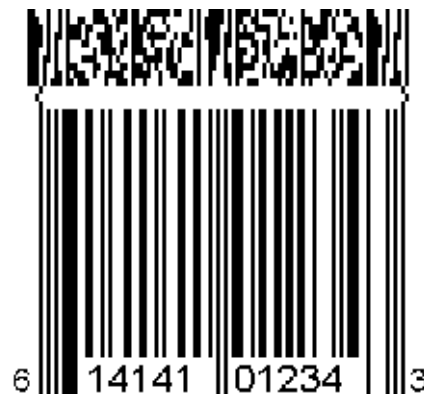
Figure 5-59 UPC-A symbol with a four-column CC-B component
