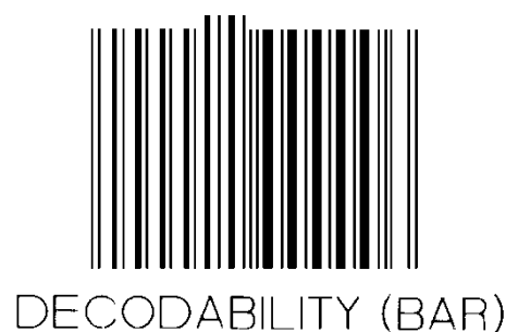
Figure 5-73 Calibration symbol with engineered low decodability grade
