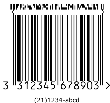
Figure 5-58 EAN-13 symbol with a four-column CC-A component
