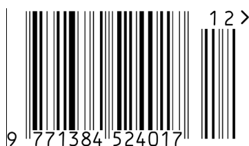
Figure 5-19 EAN-13 barcode with two-digit add-on symbol
