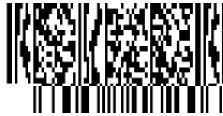
Figure 5-64 GS1 DataBar Limited symbol with a three-column CC-B
