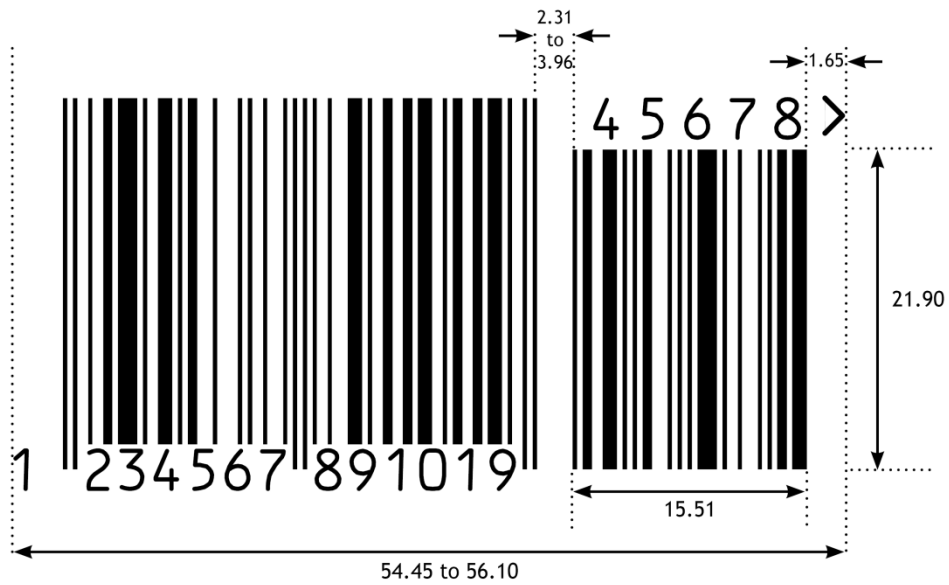
Figure 5-28 EAN-13 barcode with five-digit add-on symbol
