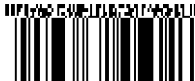
Figure 5-62 GS1 DataBar Omnidirectional symbol with a four-column CC-A
