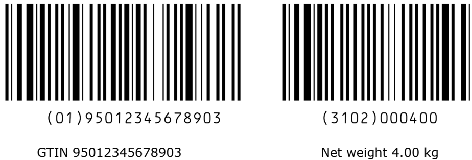
Figure 7-9 Data encoded in two GS1-128 symbols
