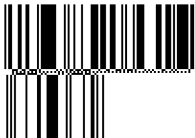
Figure 7-13 Example of GS1 DataBar Expanded Stacked barcode that uses concatenation
